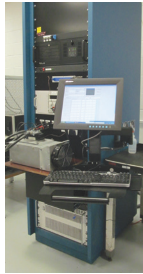
Thermal Impedance Testing
