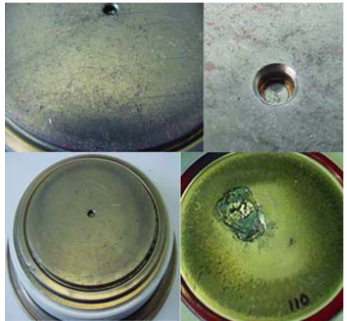
Figure 2: Failure Due to Mounting Error Exhibits Silicon Melt on Cathode
